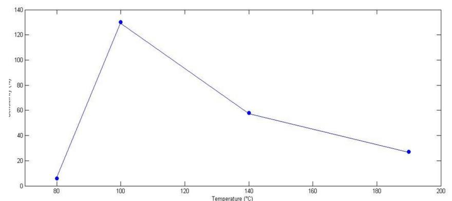
The sensitivity as a function of temperature for 10000 ppm CO in air of YCoO<sub>3</sub>
