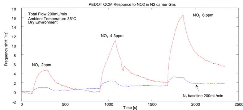
A reference baseline is obtained performing preliminary measurements in Nitrogen at 200 mL/min.
