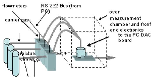
During measurements the chemical sampling and control system allows to maintain the sensors in known and predefined atmosphere and temperature. The measurement chamber allows performing measurements with 2 sensors and two reference quartzes, a humidity sensor and a temperature sensor.
