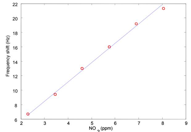
A set of 6 nominally equal sensors was tested for NO<sub>2</sub> sensitivity in the range 2 ppm-10 ppm in the same environmental conditions.
